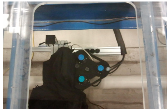
Figure 10: Location of the V3V camera probe looking from the bottom of the flume tunnel
